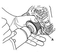
Remove the nut, pulley(A) and spacer.
