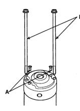
4. Remove the rear bracket (A) and brush holder assembly (B).
