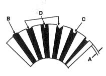
9. Check with an ohmmeter that no continuity exists between the commutator (A) and armature coil core (B), and between the commutator and armature shaft (C). If continuity exists, replace the armature.
